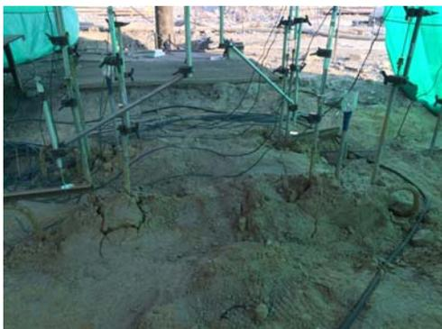
*Visible soil disturbance at ground level at the end of the O-cell test.*
