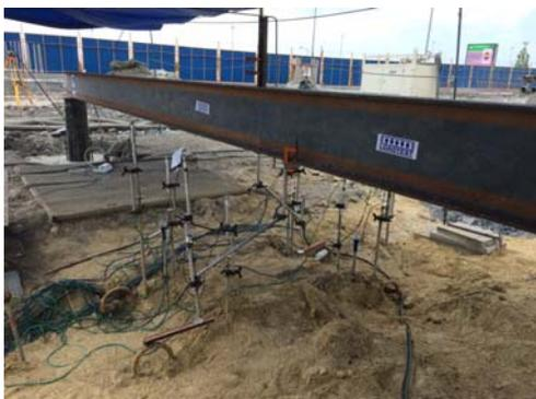
*O-Cell test setup at the top of the excavation*
