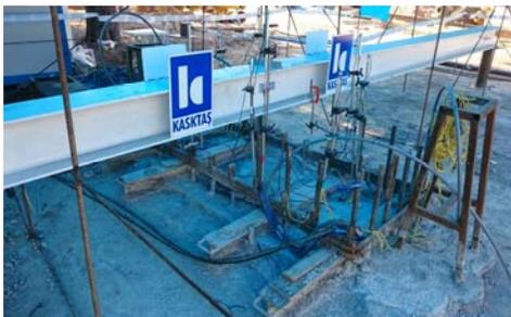
*O-Cell test setup at the top of the excavation*
